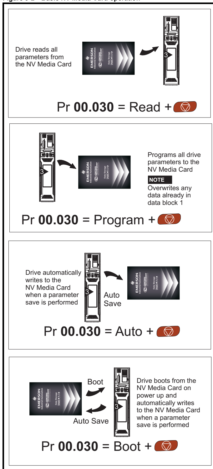
Figure 9-2 Basic NV Media Card operation
